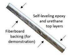
The process is odorless, and the finished floor is shiny, seamless, highly resistant to impact, and impervious to spills, chemical or otherwise, that are wiped up promptly. While many colors are available, our owner selected white, poured in subtle, flowing patterns.
